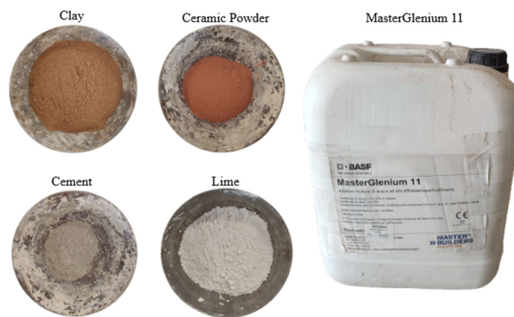
Figure 2. Materials utilized in the formulation of clay-based mixtures.
