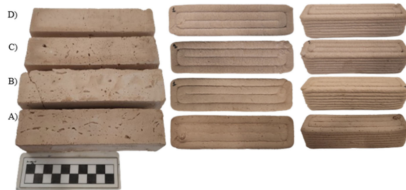
Figure 6. Final casted and 3D-printed prisms. (A) 100% Clay, (B) 95% Clay—5% Cement, (C) 90% Clay—10% Lime, (D) 80% Clay—20% Lime.
