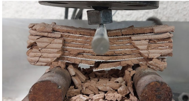
Figure 15. Flexural strength of 3D-printed specimens with reinforcing meshes tested perpendicularly to the printed layers.
