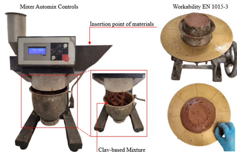
Figure 3. Preparation of clay-based mixtures.
