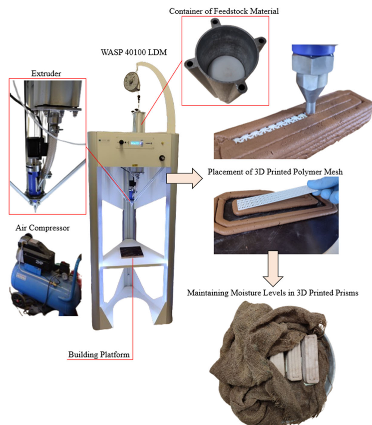
Figure 5. Three-dimensional printing of clay-based prisms.
